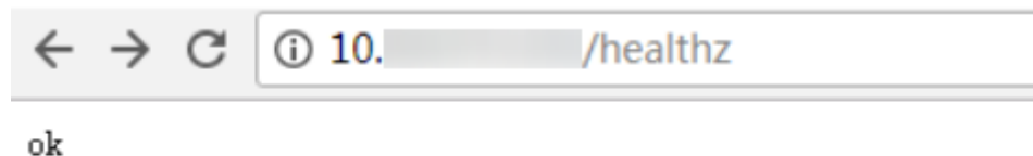
Figure 3-22 Accessing the /healthz interface of defaultbackend
